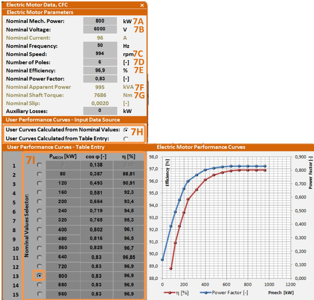
Fig.18 Frequency converter enhanced data entry
