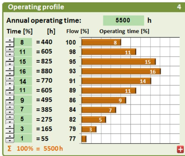
*Fig.9 Operating profile entry* because it is used for economical calculations and, thus, should not be avoided.
