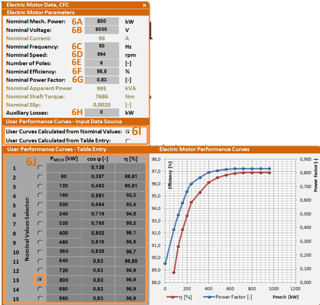
Fig.16 Enhanced motor data entry
