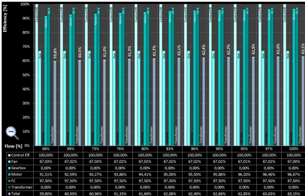
Fig.27 Enhanced Graphical Comparison - Variable Speed Control with Frequency Converter (VFC)
