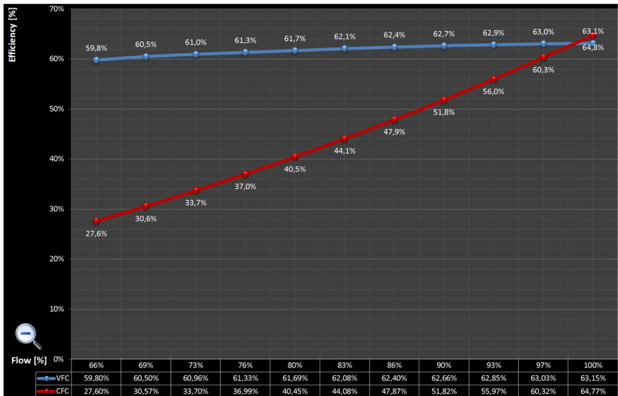
Fig.29 Enhanced Graphical Comparison – Absolute Efficiency Comparison (line graph)
