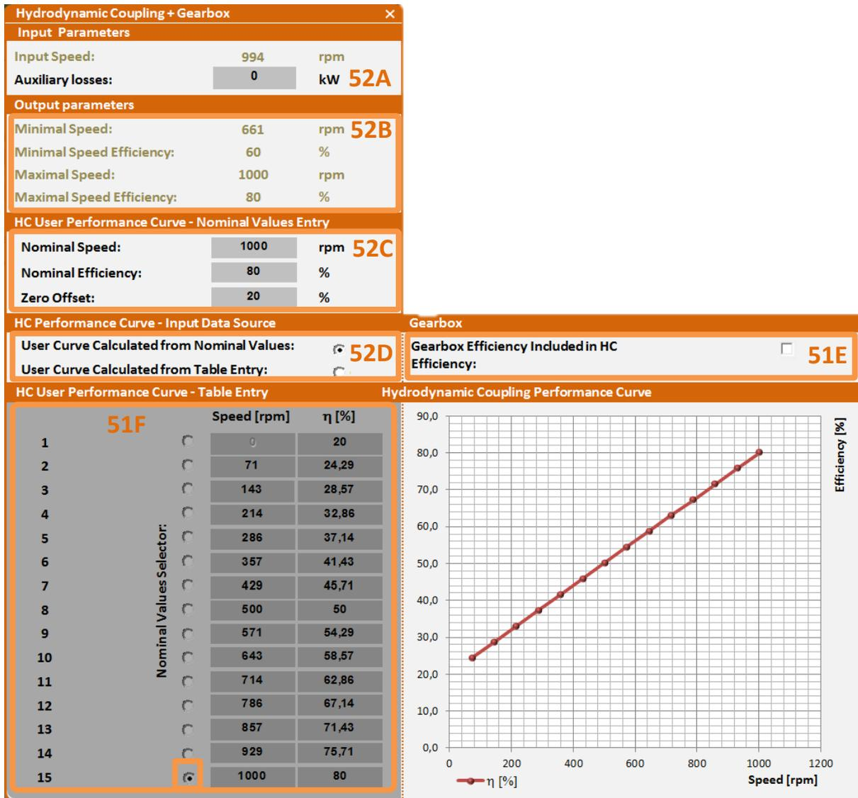
Fig.13 Enhanced Variable Speed Control – Hydrodynamic Coupling entry
